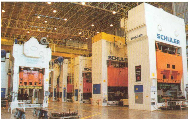
Figure 5. ES4 model Schuler presses (courtesy: General Motors).
